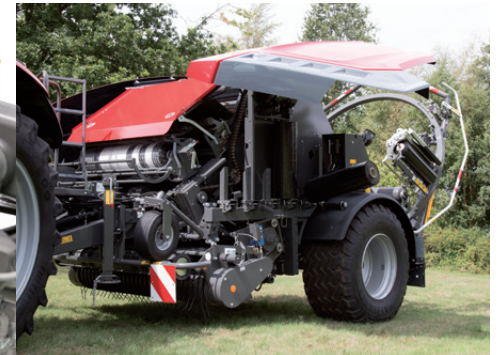
Twelve film roll holders are conveniently located at a comfortable height on both sides of the baler and with two additional rolls installed on the wrapper, increase uptime in the field.
