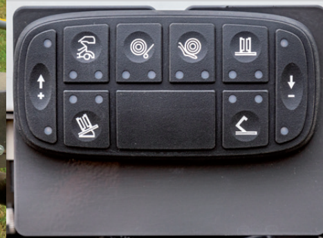
An external control panel on the back of the baler allows control of the tailgate, wrapping ring and table and the film clamps for easy film roll change, maintenance or cleaning.
