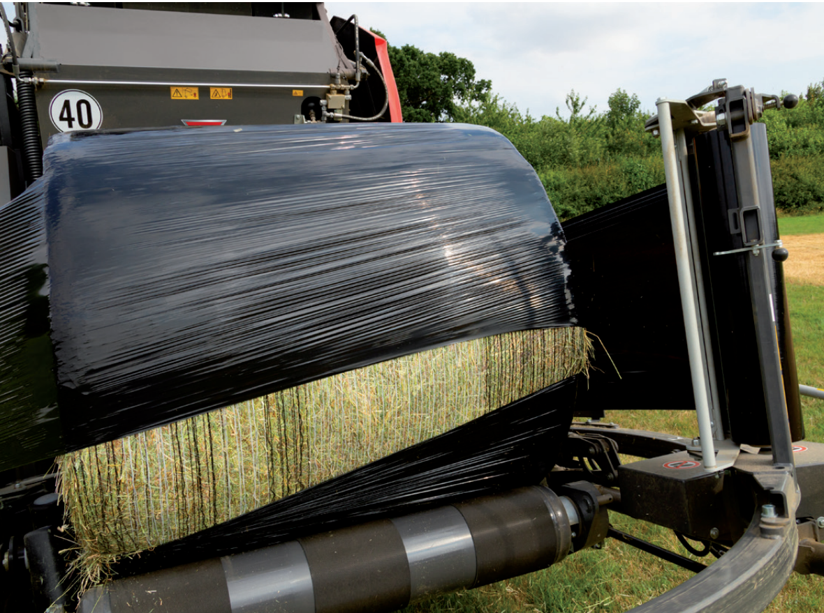
The hydraulically driven wrapper table consists of two rollers and three endless belts mounted on a welded frame for extra durability. A sensor underneath the middle belt will allow for wrapping to begin only after the bale is fully positioned on the table, while four large side support rollers keep the bale centred while wrapping.
