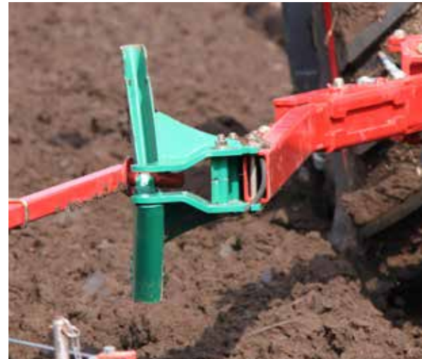
Packer arm connecting to the packer
